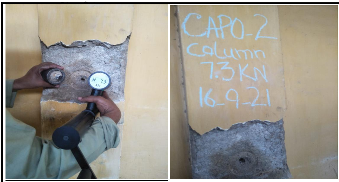
Figure-03: Peak Value of Compressive Strength is shown on Capo Gun in KN at Location -02 on
